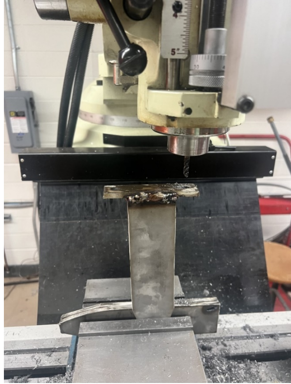
Figure 24: Milling of Holes
